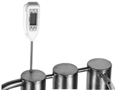
7. At 70 °C on the thermometer located on the lid of the container, start cooling, with gentle stream of water flowing through the radiator, waiting for the first condensate.
